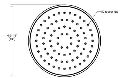
Dimensions are inches, rounded to 1/16" [Dimensions in brackets are mm, rounded to 1mm]
